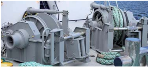
14 Units Hydraulic towing winch Vessel: Cerro Itamut Owner: Panama Canal Authority Country: Panamá
