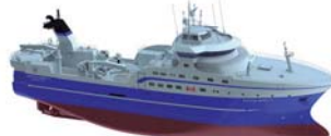
M.V. Osprey Ltd. (Canada) 80 m Factory Trawler - Electric Shipyard: Tersan - Shipdesign: Skipsteknisk
