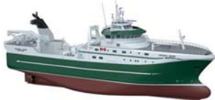
Ocean Choice International (Canada) 74 m Freezer Trawler - Electric Shipyard: Tersan - Shipdesign: Skipsteknisk
